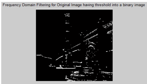
Figure 23 Frequency Domain filtering of Original image having threshold into a binary image
