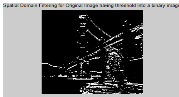
Figure 17 Spatial Domain filtering of Original image having threshold into a binary image
